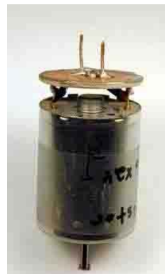
Figure 23. PCB with an X2Y® component is attached. Picture courtesy of Jastech EMC Consulting, LLC.
