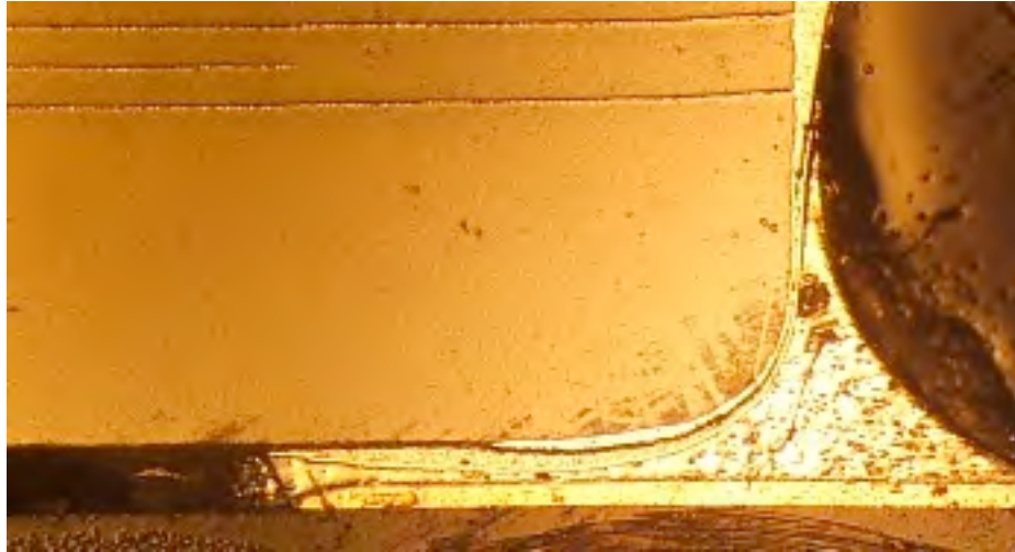
Figure 12 Partial Separation of Polymer 4mm
